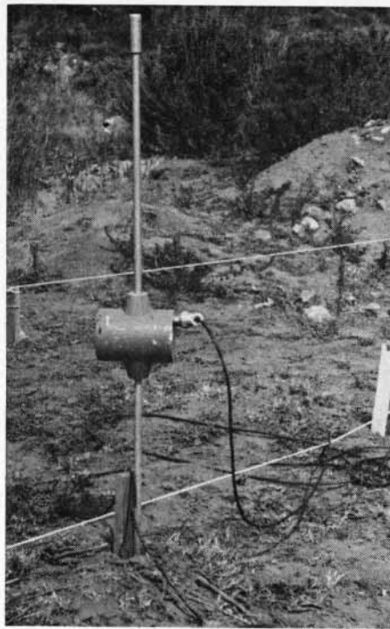
Fig. 2—The "bottle" section of a proton magnetometer.
