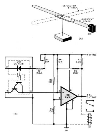
Fig. 3. Compass magnetometer's sensor (A) is a magnetic needle whose motion is sensed optically. Circuit (B) provides a TTL-compatible output and, if desired, activates a relay.
