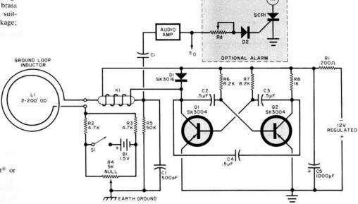
Fig. 5. Ground-loop magnetic detector responds to dc and low-frequency ac signals.
