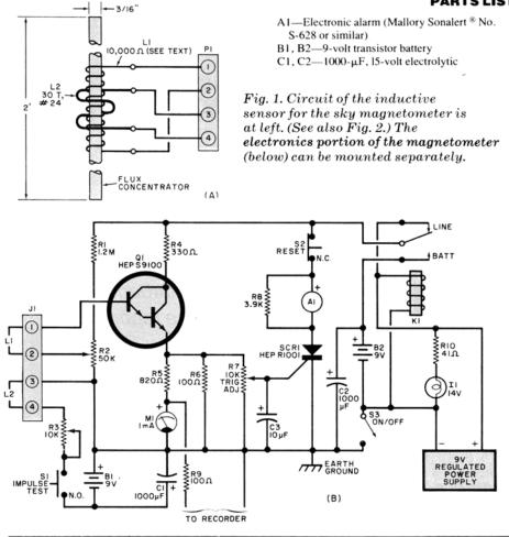
superimposed current of about 50 µA, the output of L1 amplified by Q1, will trigger the magnetometer. Near-trigger conditions can be observed on the meter, providing a built-in test facility in addition to L2.
