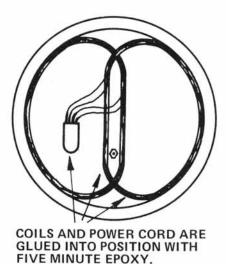
Fig. 5. Diagram showing the position of the coils in the search head.
