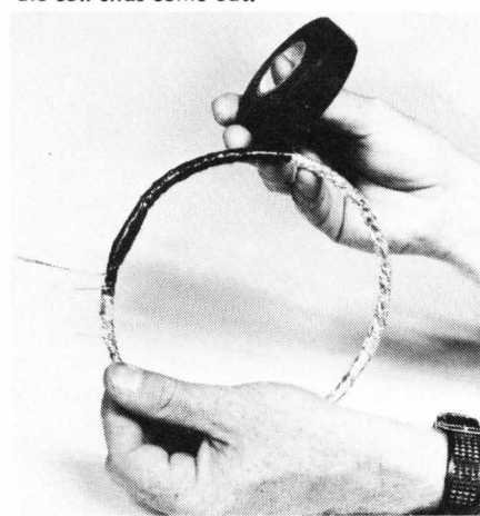
4: Cover the whole coil assembly with two more layers of insulation tape.
