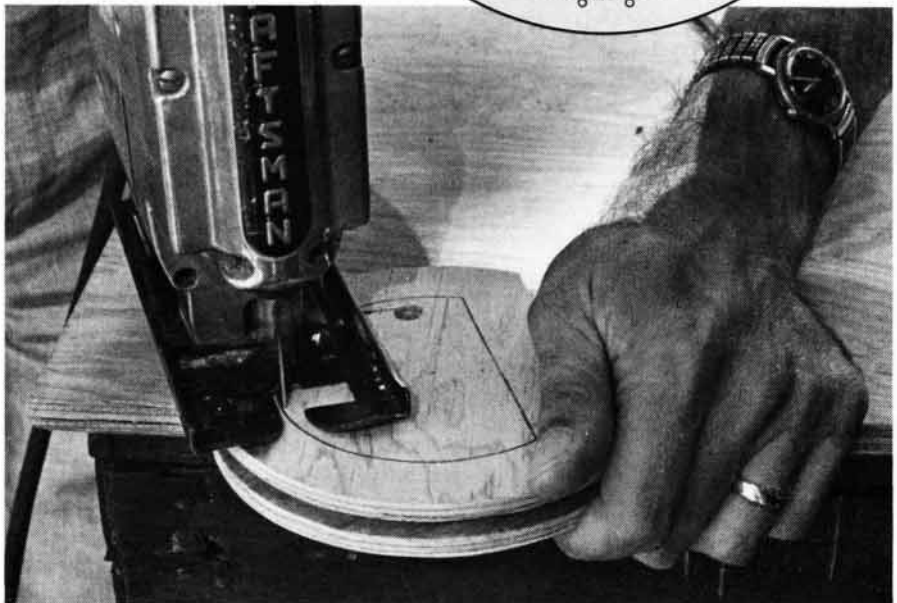
Fig. 5. Use a coping or sabre saw to cut out the form drawn on disc in Fig. 4.
