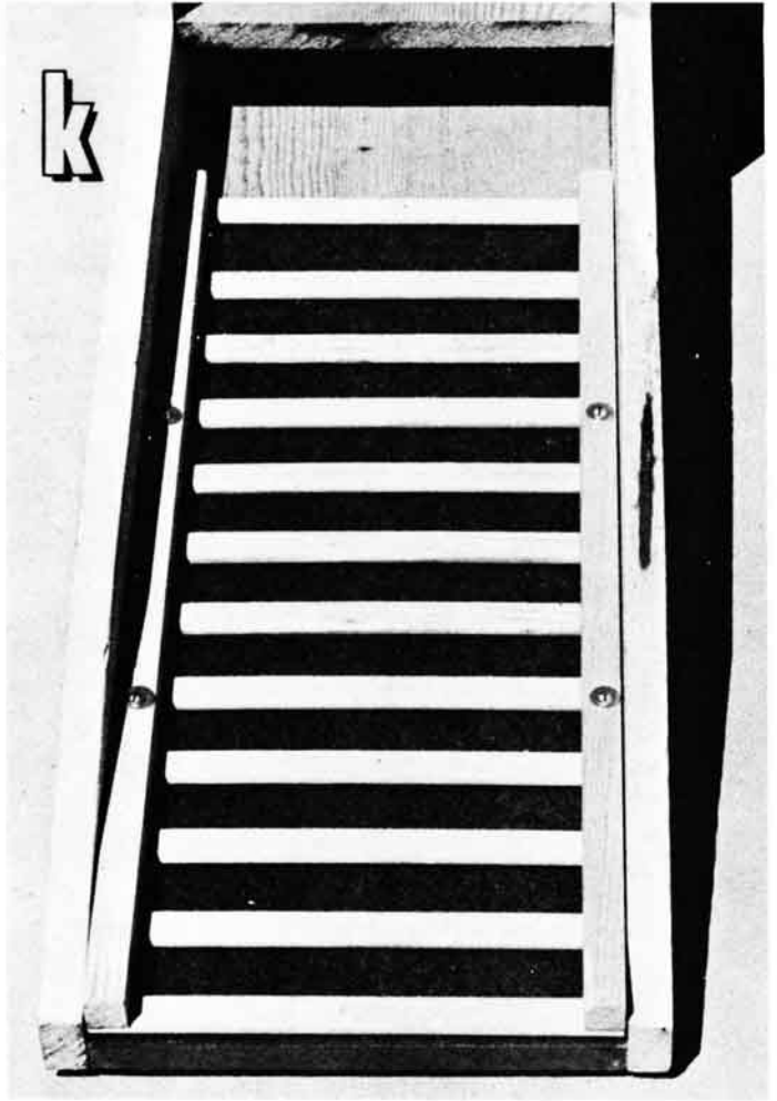
The last step is to position the carpeting and riffle tray in the main box, then drill four 1/4 inch holes through the 1x1's, the carpeting, and the bottom of the main box. Install the bolts, which ensure that the riffles are held down firmly against the carpeting.
