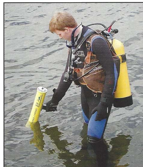
Tracking Cable in Shallow Water
