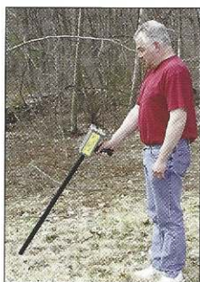
Tracking an armored cable on land
