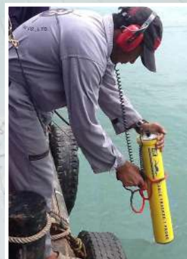
CT-1 used to help find & track damaged cables
