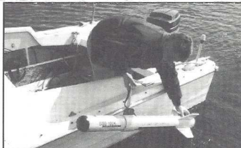
EASY DEPLOYMENT OF SIDE SCAN FISH
