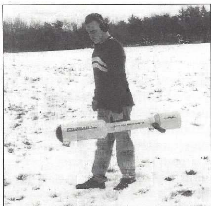
SEARCHING FOR A BURIED PIPELINE WITH FISHERS NEW DIVER MAG 1
