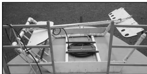
SITTING ON THE FRONT OF MIKE'S BOAT IS HIS CUSTOM SLED WITH THE PULSE 10 COIL ATTACHED TO BOTTOM
