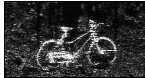
Image of bicycle on river bottom produced by Fishers SSS-1200 kHz side scan sonar
