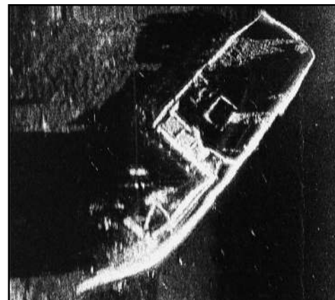
Side scan image of sunken vessel
