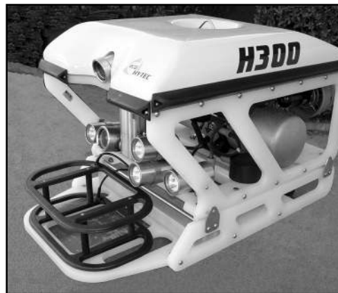
ECA Robotics ROV with Fishers RMD-1 remote metal detector mounted on front
