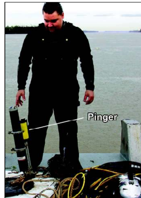
Commercial diver with recovered ADCP with attached JW Fishers SFP-1 pinger
