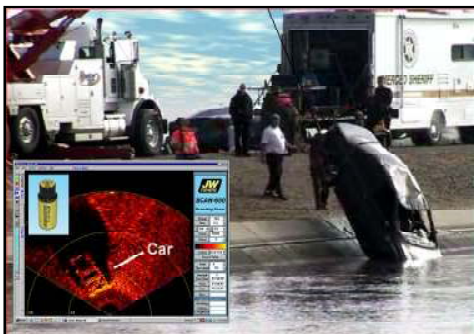
Car being pulled from drainage canal, Inset - Sonar image of car on bottom
