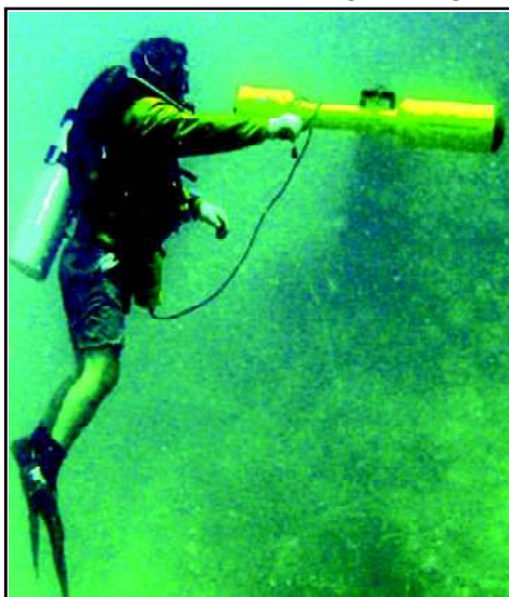
Diver scans reef for magnetic anomalies with Fishers Diver Mag magnetometer
