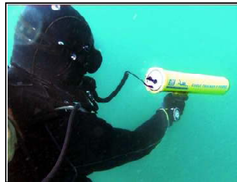
Diver scans area with CT-1 cable tracker
