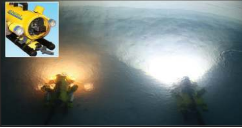
Old 100 watt halogen lights (L) compared to new 2200 lumen LED lights (R) on ROV
