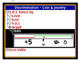
The displayed number shows the VDI number you are editing. Also shown are the icons that are set for that VDI. Use the  $\triangleleft$  and  $\triangleright$  buttons to move left and right through the VDI range, and the  $\triangle$  and  $\blacktriangledown$  buttons to accept and reject (respectively) the selected VDI.
