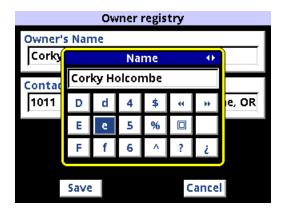
Use **AV** to move around the keyboard; press **ENTER** to "type" the selected key; when you are done, pull the trigger switch to exit back to the registry screen.
