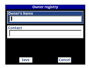
You may now enter your name, press **TAB**, and enter your contact details. Use the  $\triangle$  and  $\bigvee$  keys to select characters, and the  $\triangleleft$  and  $\bigvee$  keys to move backwards and forwards in the edit window. You may also press **ENTER** to access the *V3i* **Keyboard Editor**, which is covered in detail in the last part of this chapter.
