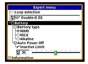
With **Battery type** you can select which battery pack you are using, and V3i will slightly tweak the battery graphic on the splash screen. However, for most people this is not an important consideration so leaving the battery type set to a single entry is fine.
