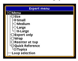
Out of the box, V3i has the 6-block menus enabled and easily accessed, while the Expert Menus take several key strokes to enter. As you gain experience using V3i, you may want to replace the 6-block menus with the Expert Menus. The above option **Expert Only** does this; when you check this option, a press of the **MENU** key during normal search will bring up the Expert Menus instead of the 6-block menus.
