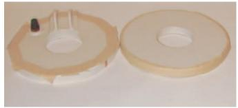
Fig 7: Shells masked for nickel spray
