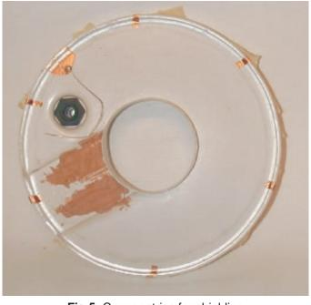
Fig 5: Copper strips for shielding
