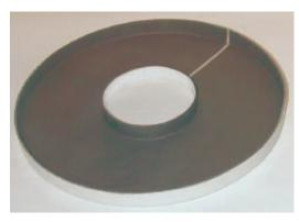
Fig 10: Small gap in the shield
