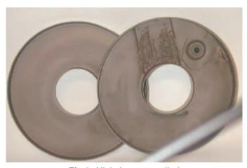
Fig 9: Nickel spray applied
